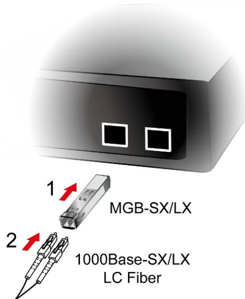
Figure 2-1-2e Plug in the SFP transceiver
