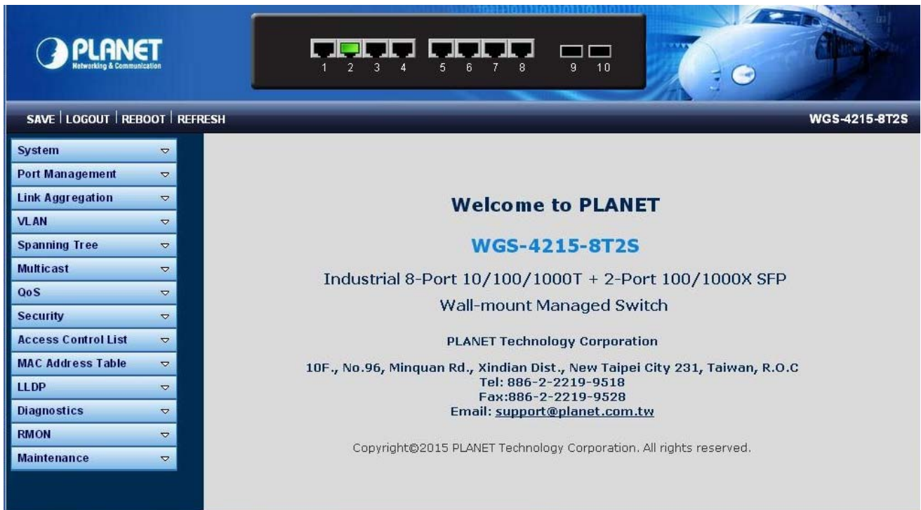
Figure 3-1-2 Web Main Screen of Managed Switch
