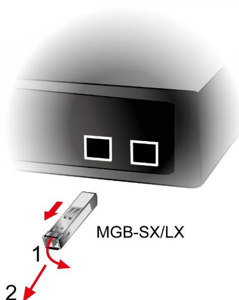
Figure 2-1-2f How to Pull Out the SFP Transceiver
